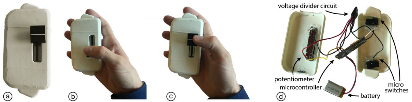
Figure 3: a) BASIC SLIDER, b) minimum value, c) maximum value, and d) electronic components including microcontroller, battery, potentiometer, voltage divider circuit, and micro switches.
