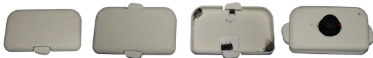
Figure 1: Various prototypes exploring the type, size, and placement of confirmation buttons. Right photo shows the final design with large button covers mounted to micro switches, fixed at the midpoint of the top and bottom edges (shown here for ANALOGUE STICK).
